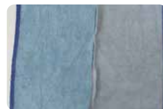
Figure 3 - Comparison of blue microfibre cloths after multiple exposures to Surfex® (left) or Chlorine based product (right)
