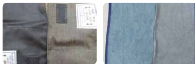
Figure 2 - Comparison of Sphygmomanometer test articles after multiple exposures to Surfex® (left) or Chlorine based product (right)
